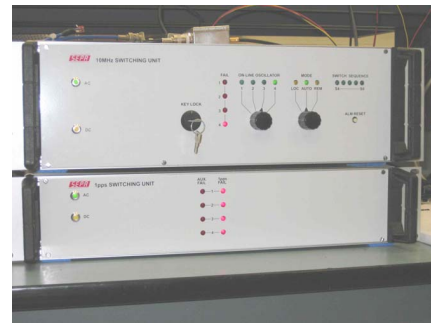
Figure 9. Automatic Switching Matrix under test at SEPA
